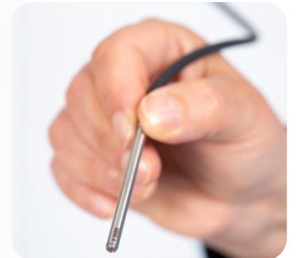
Successfully miniaturised high resolution benchtop confocal microscope into hand-held probe with 4.0mm diameter providing unique microscopic imaging for clinicians. Underpinned by multi-patented technology.
