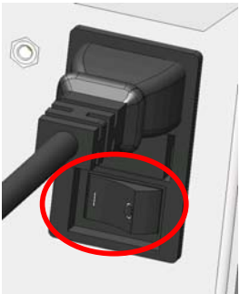
Turn the Viewvivo Processor Main Power ON
