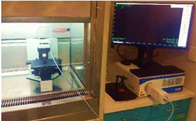
A prototype set up: Optiscan's FIVE2 confocal endomicroscope probe set up inside the biosafety cabinet for imaging tissue culture.
